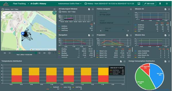
History tracing is a dedicated dashboard with feature to select any desired time period in mission or vessel operational history and all recorded data will be visualized. The data can also be traced by location and mission can be fully replayed. All data can be exported as raw, directly from the server in a form of csv files.
