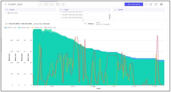
The recorded data has a limited value if the desired insights are not retrieved from it. The data analytics module is doing exactly this. It is featured with predefined or custom algorithms for data aggregation, anomaly detection and forecasting. The algorithms range from simple square methods to advanced AI anomaly detection methods.
