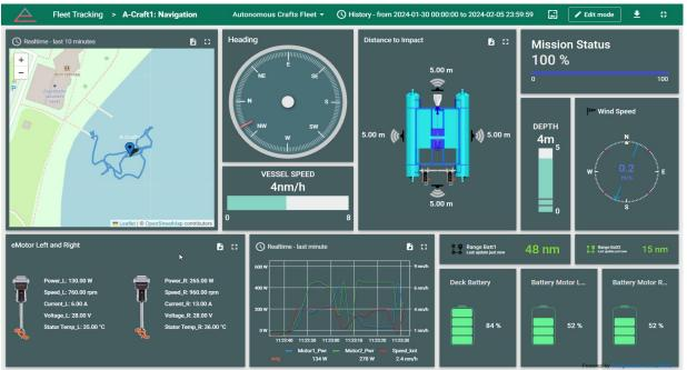
Navigation window is a vessel performance monitoring dashboard. It shows information such as heading, route, vessel speed, depth, distance to impact, wind speed and direction, deck and engine battery status, eMotor current, voltages, temperatures, power and speed. It also has graphical view of relation between eMotor power to speed and heading.
