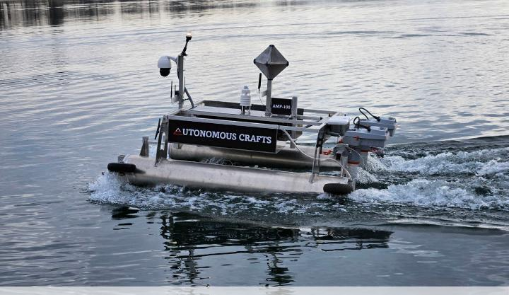
AMP-100 can conduct surveys with different levels of **autonomy** (**M**, **DS**, **DSE**, **SC**) and sends real-time data of utility sensors, cameras, propulsion, batteries and navigation onto the remote operations station. The data is processed and plotted in real-time, history and analytics form in a single or fleet mode within our **data platform**.
